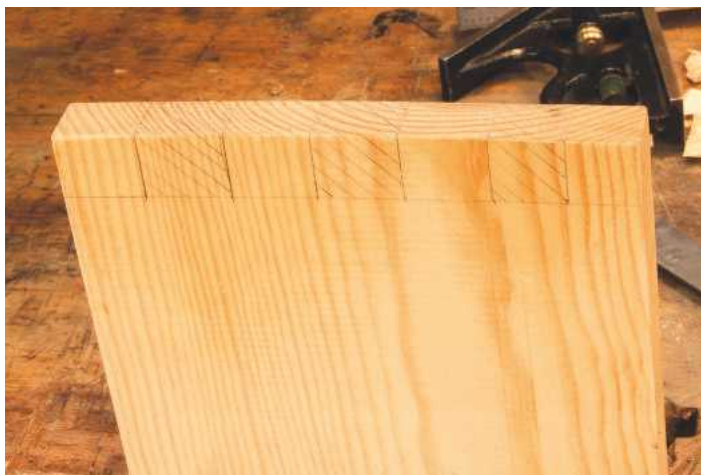
▲ Pic.8 Finger joints marked up – good practice for dovetailing
